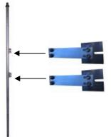
Step 17: Insert the rotation shaft assembly into the HEPA filter. It will be easier to insert while holding it at an angle. Insert the bottom end of the shaft into the hole in the bottom of the filter.
