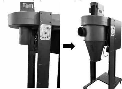
Step 10: Secure the filter cover using (4x) 1/4"x3/4" bolts and (4x) 1/4" washers.
