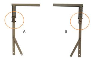
Step 25: Slide the bar into the opening on the lower upright support. Follow the same steps for the opposite side.
