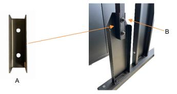
Step 28: Cover the lifting mechanism with lower cover plates. Secure using (6x) 1/4"x3/4" hex bolts and (6x) 1/4" washers. Follow the same steps for the opposite side.
