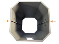
Step 39: On the left and right side of the drum you will find three bolt holes. Secure the matching side plate to the drum panel using (6x) 1/4"x1/2" bolts, (6x) 1/4" washers and (6x) 1/4" nuts. Insert the head of the bolt from the inside of the drum with the washers and nuts on the outside of the drum.
