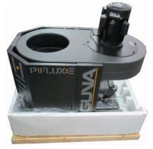
Step 2: Remove base frame that is bolted to (3x) top upright supports. Keep (6x) 3/8"x3/4" bolts and (6x) 3/8" washers.
