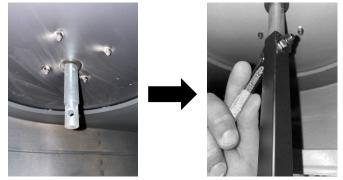
Step 19: Tighten the (1x) 5/16"x3/4" screw and (1x) 5/16" washer on the bottom of the rotation shaft.
