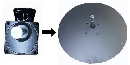
Step 14: Take the hardware removed in step 12 to fasten the Autoclean motor to the plate. Thread the bolts on the Autoclean motor side (A) and the nuts on the plate side (B). Do not fasten the bolts and nuts the other way round.
