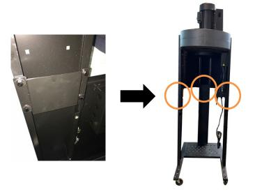
Step 7: Take the junction box and secure it to the reinforcement plate beneath the control panel using (2x) 1/4"x3/4" bolts and (2x) 1/4" washers.
