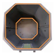
Step 43: Attach the rubber gasket to the top rim of the drum. Remove excess rubber gasket.
