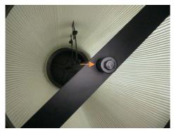
Step 20: Open the filter shield and secure the HEPA filter to the dust chute by fastening the band clamp on the top part of the filter. Make sure the band clamp is tightly fastened.
