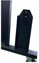
Step 23: Secure the lifting mechanism support to the lower upright support using (2x) 5/16"x1/2" bolts, (2x) 5/16" washers and (2x) 5/16" nuts.
