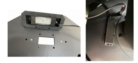
Step 35: Attach the crossbar to the drum lid and tighten using (2x) 5/16"x3/4" bolts, (4x) 5/16" washers and (2x) 5/16" nuts. It does not matter which position you attach the crossbar.
