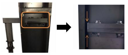
Step 27: Secure the U-channel (A) to the triangular support plate using (2x) 5/16"x1-3/4" bolts, (4x) 5/16" washers and (2x) 5/16" nuts so that the bolt head is on the inside (B). Follow the same steps for the opposite side.
